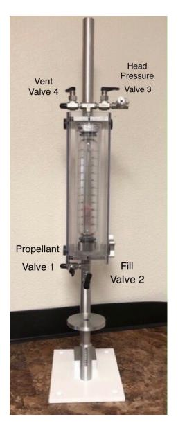
First fully read and understand the operating instructions, safety precautions and warning sheets supplied **before you operate!!** Then level and fasten your pressure filler to the surface it is being used on with the fasteners supplied. Your propellant line would go to valve 1. Your head pressure would go to valve 3. Valve 4 is your vent and valve 2 is where you attach your valve adapter.
